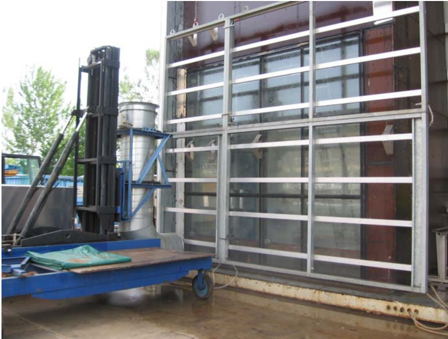
Fig. 3 Facade with spray grid suspended in front for watertightness test, at left fan for dynamic watertightness test
