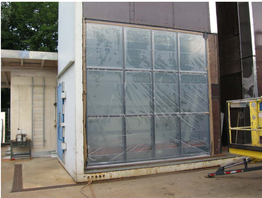
Fig. 2 Facade with film suspended in front for zero measurement
