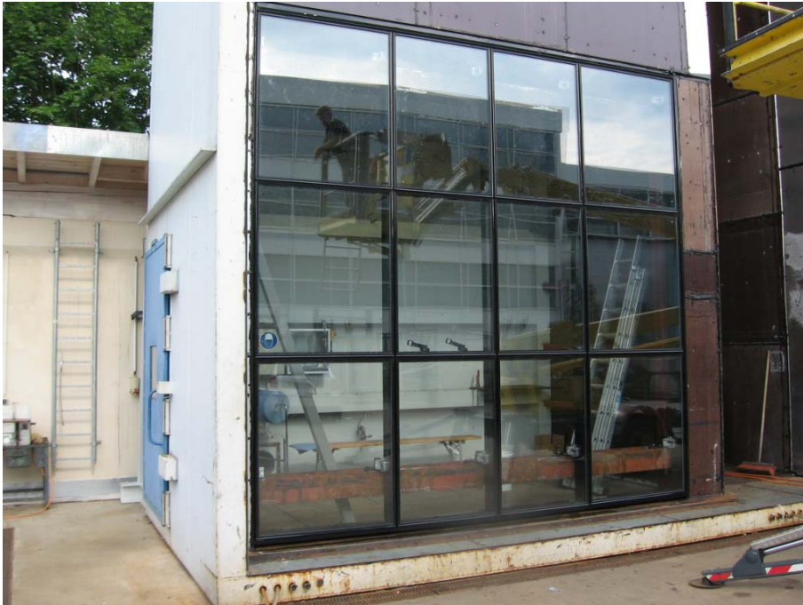
Fig. 1 Facade mounted to test rig
